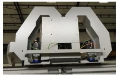
The motion of the carriage running on the crossbeam, transversal axis  $\hat{I} \times \hat{I}$ , is also managed by 2 servomotors.
